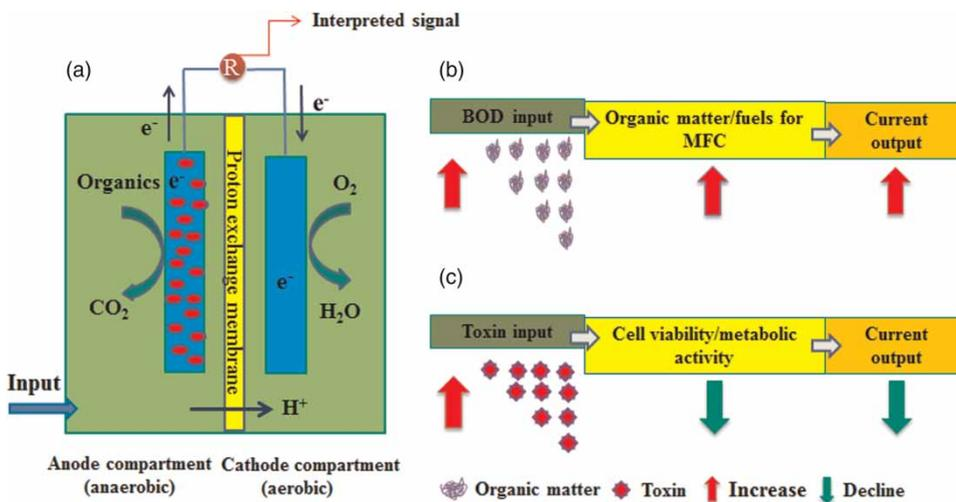
**Figure 2** | (a) Schematic diagram of an MFC. (b) Mechanism for MFC-based BOD monitoring. Increased BOD input provides more organic matter/fuel for the MFC, which in turn results in an increase in current output. (c) Mechanism for MFC-based toxicity monitoring. Increased toxin input will repress/inhibit the cell viability/metabolic activity, which directly reduces the current output.
