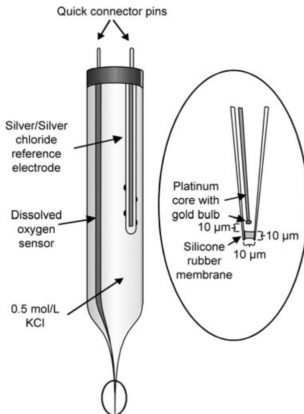
**Fig. 1** Dissolved oxygen microelectrode (DOM). Reproduced from Lewandowski and Beyenal (2007).
